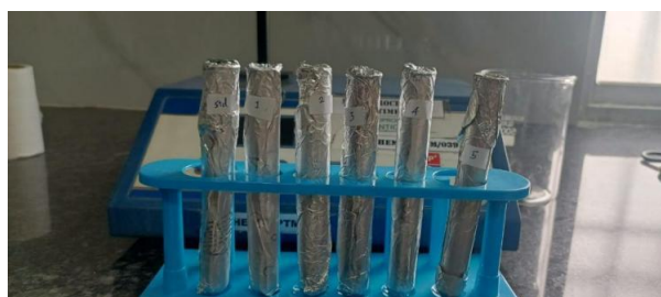
Fig.7: Test tube containing sample and DPPH
