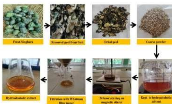
Fig. 1. Flow chart representing the preparation process of 50% hydroalcoholic extract from T. natans L. peel.
